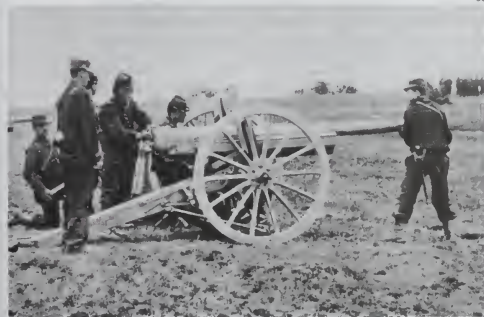
Figure 15. The French 75-millimetre cannon of 1897. With screw-threaded breech, hydropneumatic recoil control, and metallic-cartridge ammunition, this was the archetypal quick-firing gun of the late 19th and early 20th centuries.
